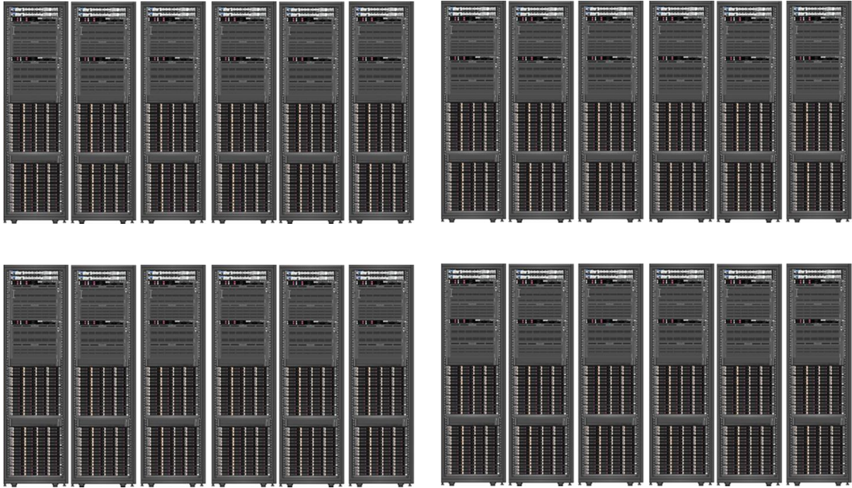
EDMT® Solution Model 4K (48x HP DL 980, 3,840 cores, 10 PB)
