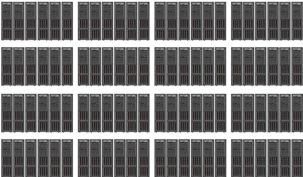
EDMT® Solution Model 16K (192x HP DL980, 15,360, 40 PB)
